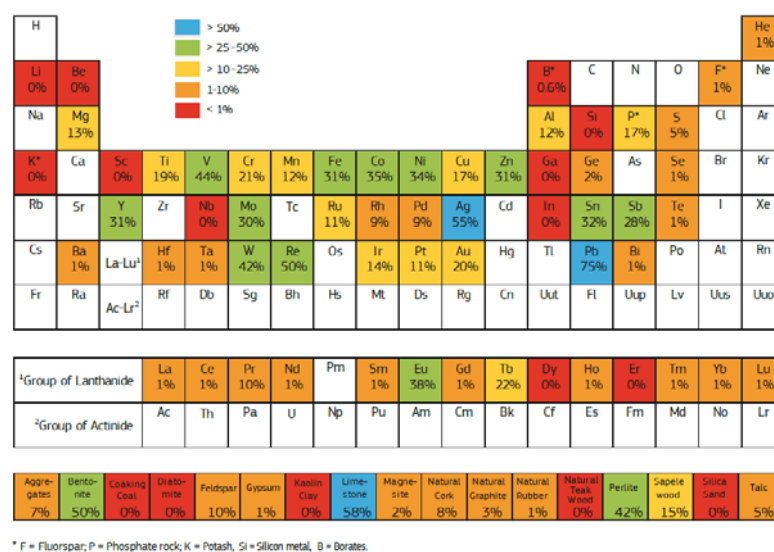
Figure 21. End-of-life recycling input rate (%) to contribute to the EU demand of CRMs (Beatriz et al., 2018; Blengini et al., 2019)
